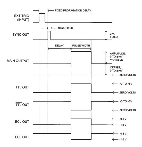
As before, if the delay mode is set to "MAIN OUT ADVANCED", the order of the SYNC and OUT pulses is reversed.
