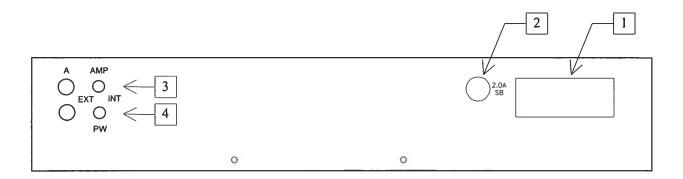
1. <u>AC POWER INPUT</u>. A three-pronged recessed male connector is provided on the back panel for AC power connection to the instrument. Also contained in this assembly is a slow-blow fuse and a removable card that can be removed and repositioned to switch between 120V AC in and 240V AC in.
