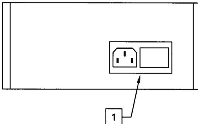
1. **AC POWER INPUT.** A three-pronged recessed male connector is provided on the back panel for AC power connection to the instrument. Also contained in this assembly is a slow blow fuse and a removable card that can be removed and repositioned to switch between 120V AC in and 240V AC in.
