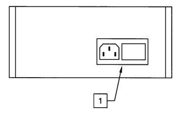
1. <u>AC POWER INPUT</u>. A three-pronged recessed male connector is provided on the back panel for AC power connection to the instrument. Also contained in this assembly is a slow blow fuse and a removable card that can be removed and repositioned to switch between 120V AC in and 240V AC in.
