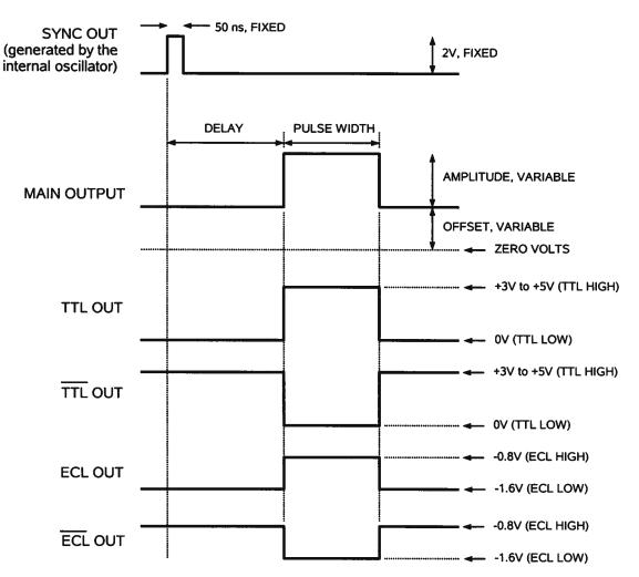
The next figure illustrates the relationship between the signals when an external TTLlevel trigger is used (i.e., the REPETITION RATE switch is set to "EXT"):
