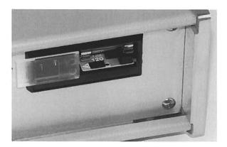
For AC line voltages of 220-240V, the power selector card should be installed so that the "240" marking is visible from the rear of the instrument, as shown below:
