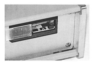
If it is not set for the proper voltage, remove the fuse and then grasp the card with a pair of pliers and remove it. Rotate horizontally through 180 degrees. Reinstall the card and the correct fuse.
