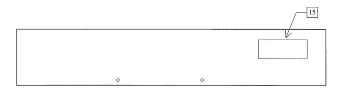
15. <u>AC POWER INPUT</u>. A three-pronged recessed male connector is provided on the back panel for AC power connection to the instrument. Also contained in this assembly is a slow blow fuse and a removable card that can be removed and repositioned to switch between 120V AC in and 240V AC in.
