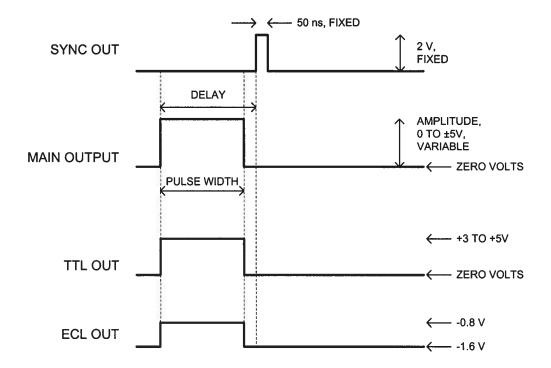
The next figure illustrates the relationship between the signals when an external TTL-level trigger is used (i.e., the REPETITION RATE switch is set to "EXT"), assuming that the delay mode is set to "MAIN OUT DELAYED":
