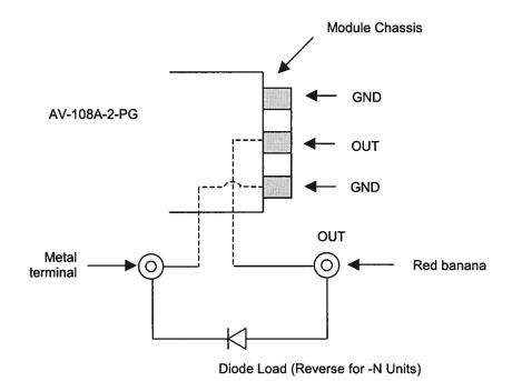
The load should be connected between the OUT and GND terminals using very short leads ( $\leq$  10.0 cm). If the load cannot be placed directly on the output terminals of the -PG module, the AV-LZ lines should be used between the -PG module and the load (see AV-LZ data sheet).
