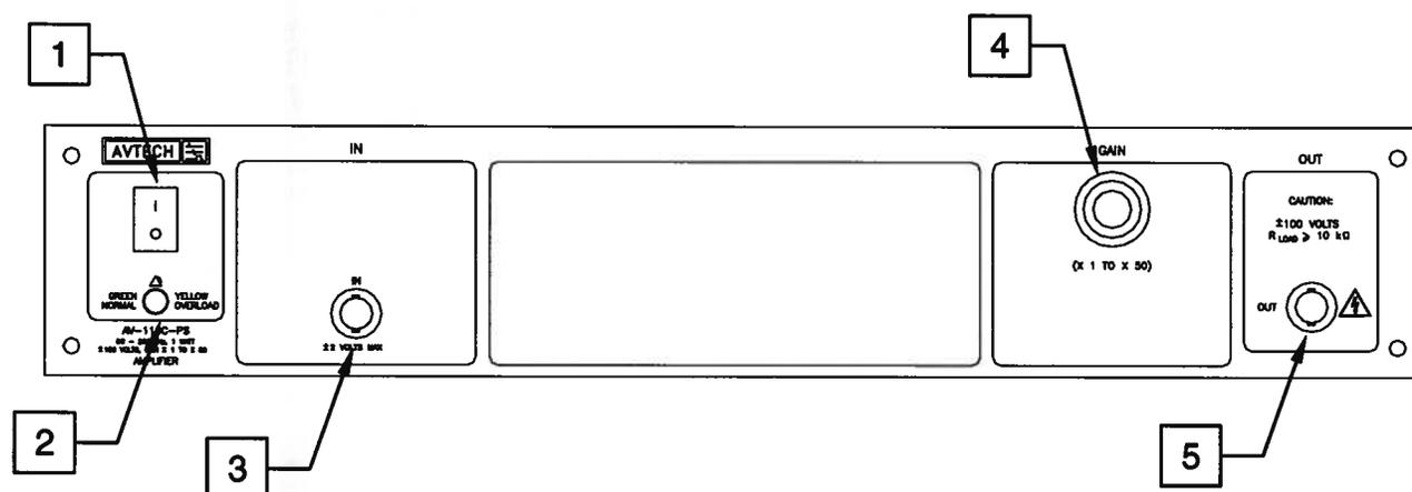
1. **POWER Switch.** This is the main power switch. When turning the instrument on, there may be a delay of several seconds before the instrument appears to respond.
