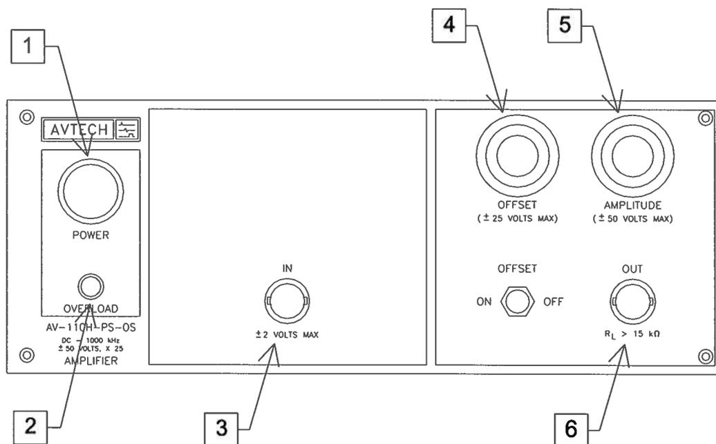
1. **POWER Switch.** The POWER push button switch applies AC prime power to the primaries of the transformer, turning the instrument on. The push button lamp is connected to the internal +15V DC supply.
