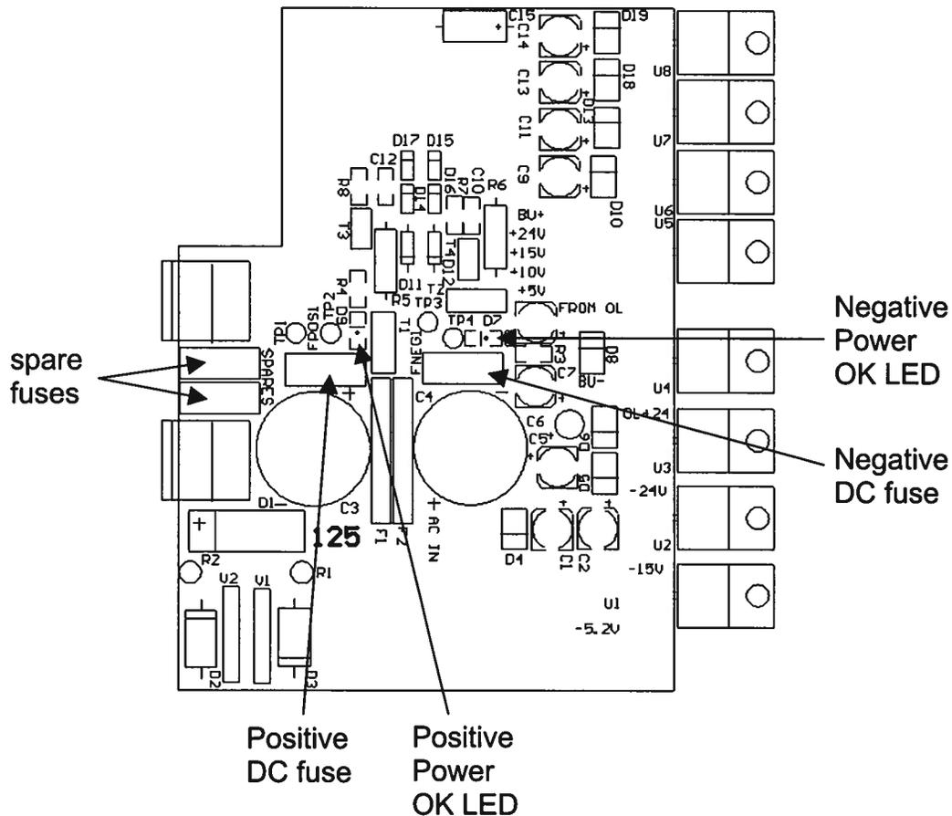
The positive fuse and one of the spare fuses on this circuit board are 1A slow-blow fuses, Littelfuse part number R452001. (This fuse can be ordered from Digikey, [www.digikey.com](http://www.digikey.com). The Digikey part number is F1343CT-ND). The negative fuse and the second spare fuse are 0.5A slow-blow fuses (Littelfuse R452.500, Digikey part number F1341CT-ND).
