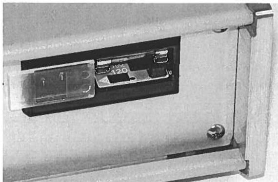
For AC line voltages of 220-240V, the power selector card should be installed so that the "240" marking is visible from the rear of the instrument, as shown below:
