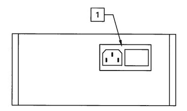
1. <u>AC POWER INPUT</u>. A three-pronged recessed male connector is provided on the back panel for AC power connection to the instrument. Also contained in this assembly is a slow-blow fuse and a removable card that can be removed and repositioned to switch between 120V AC in and 240V AC in.
