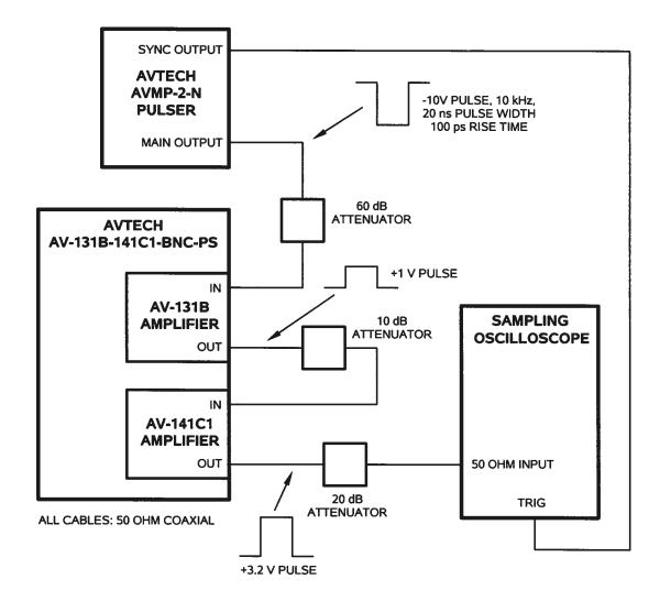
The test set-up used at the factory is shown above.
