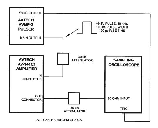
The recommended test set-up is shown above.
