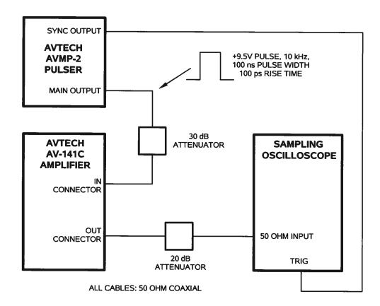
The recommended test set-up is shown above.
