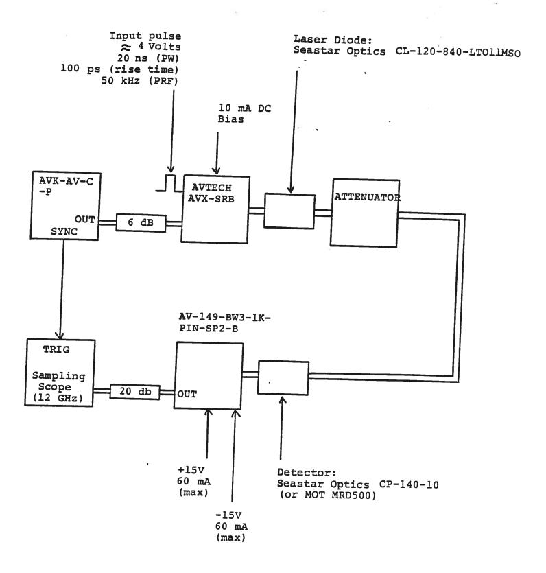
Fig. 1 BASIC TEST SET-UP (PULSE MODE)
