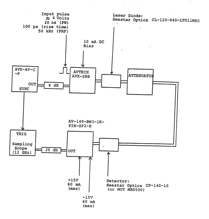
Fig. 1 BASIC TEST SET-UP (PULSE MODE)
