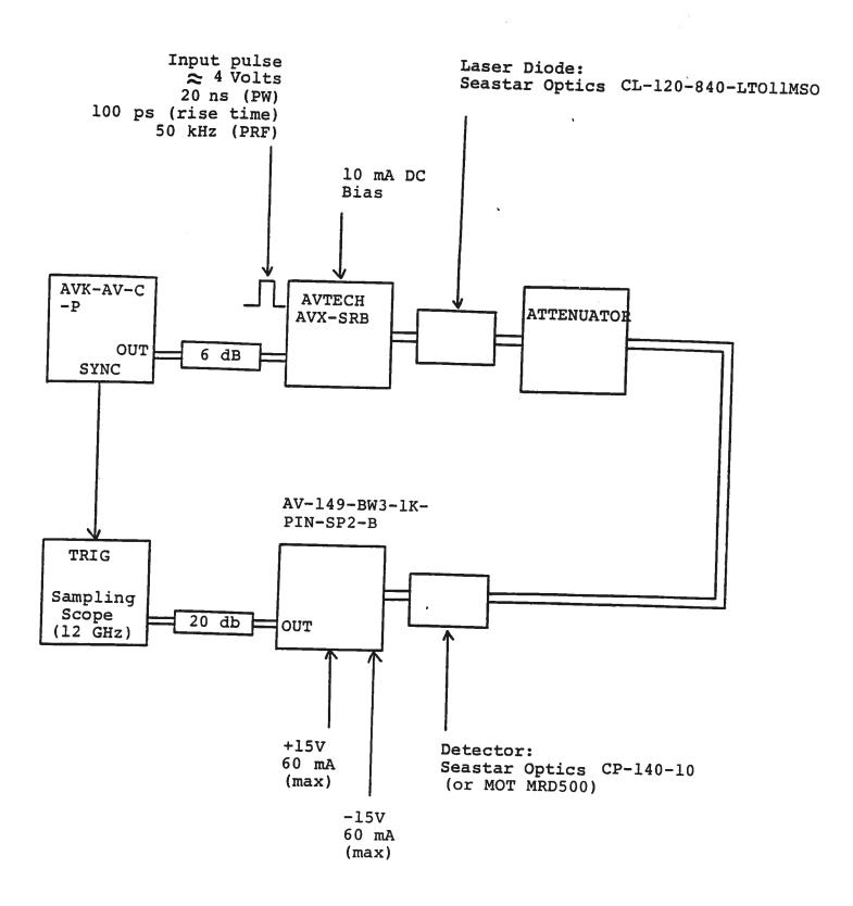
Fig. 1 BASIC TEST SET-UP (PULSE MODE)
