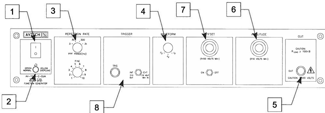
1. **POWER Switch.** The POWER push button switch applies AC prime power to the primaries of the transformer, turning the instrument on. The push button lamp is connected to the +15V DC supply.
