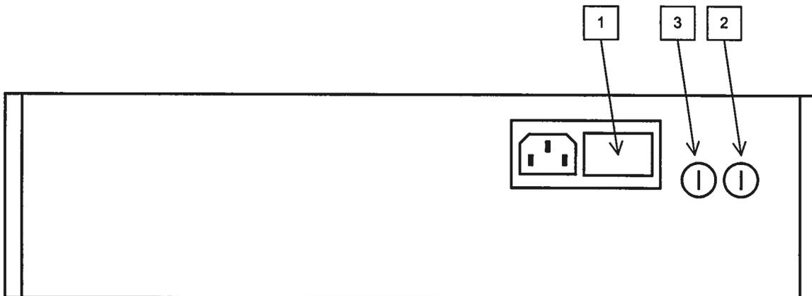
1. AC POWER INPUT. A three-pronged recessed male connector is provided on the back panel for AC power connection to the instrument. Also contained in this assembly is a slow-blow fuse and a removable power selector card that can be removed and repositioned to switch between 110-120V AC in and 220-240V.
