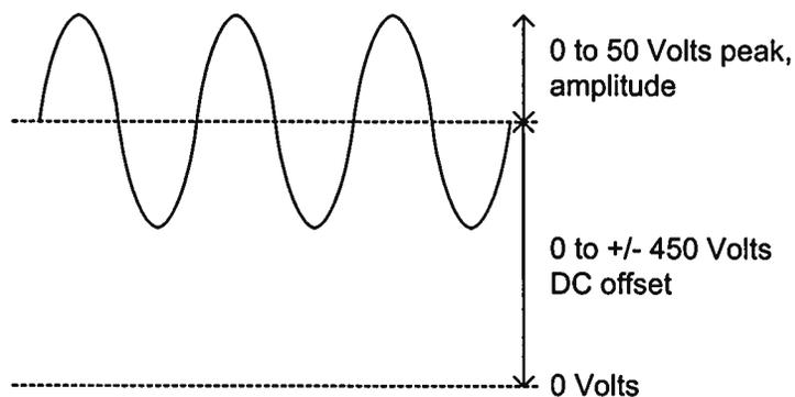
The total output (i.e., the sum of the offset and the amplitude) may not exceed  $\pm 500V$ .
