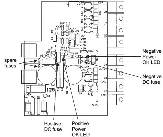
The positive fuse and one of the spare fuses on this circuit board are 1.5A slowblow fuses, Littlefuse part number R45201.5. (This fuse can be ordered from Digikey, www.digikey.com. The Digikey part number is F1344CT-ND). The negative fuse and the second spare fuse are 0.5A slow-blow fuses (Littlefuse R452.500, Digikey part number F1341CT-ND).
