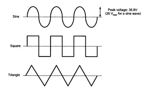
The minimum load resistance is 65 Ohms. The output signal may be obtained from the front or rear connectors, as desired.
