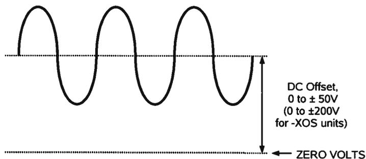
The total output (i.e., the sum of the offset and the amplitude) may not exceed  $\pm 200\text{V}$ .
