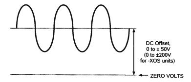
The total output (i.e., the sum of the offset and the amplitude) may not exceed ±200V.
