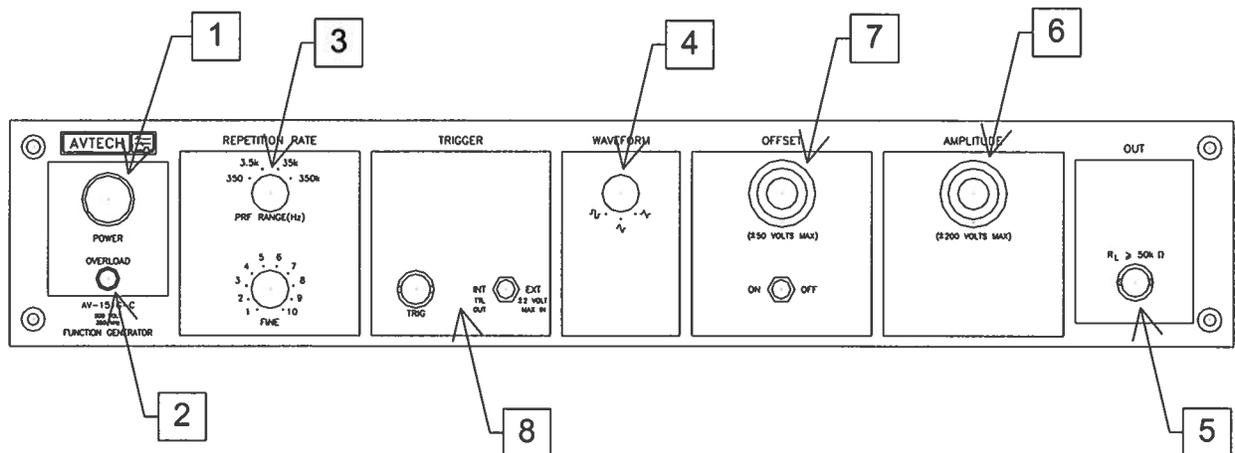
1. **POWER Switch.** The POWER push button switch applies AC prime power to the primaries of the transformer, turning the instrument on. The push button lamp is connected to the +15V DC supply.
