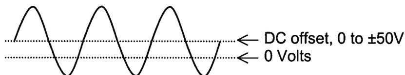
The total output (i.e., the sum of the offset and the amplitude) may not exceed  $\pm 200V$ .
