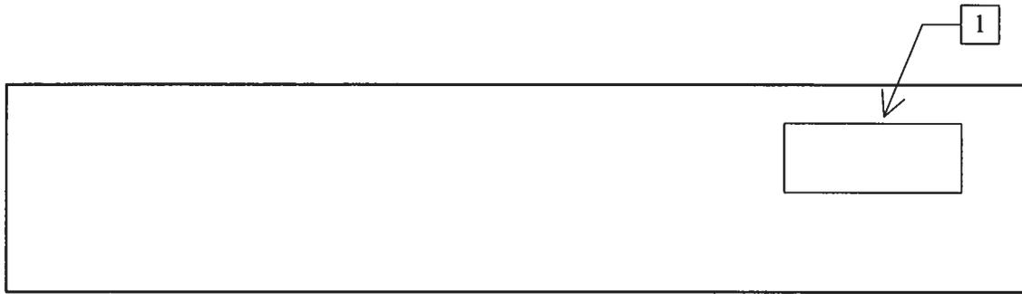
1. AC POWER INPUT. A three-pronged recessed male connector is provided on the back panel for AC power connection to the instrument. Also contained in this assembly is a slow-blow fuse and a removable power selector card that can be removed and repositioned to switch between 110-120V AC in and 220-240V.
