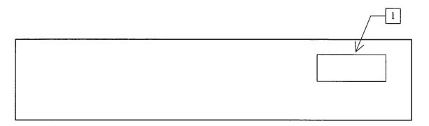
1. <u>AC POWER INPUT</u>. A three-pronged recessed male connector is provided on the back panel for AC power connection to the instrument. Also contained in this assembly is a slow-blow fuse and a removable power selector card that can be removed and repositioned to switch between 110-120V AC in and 220-240V.
