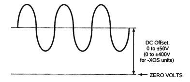
The total output (i.e., the sum of the offset and the amplitude) may not exceed ±400V.
