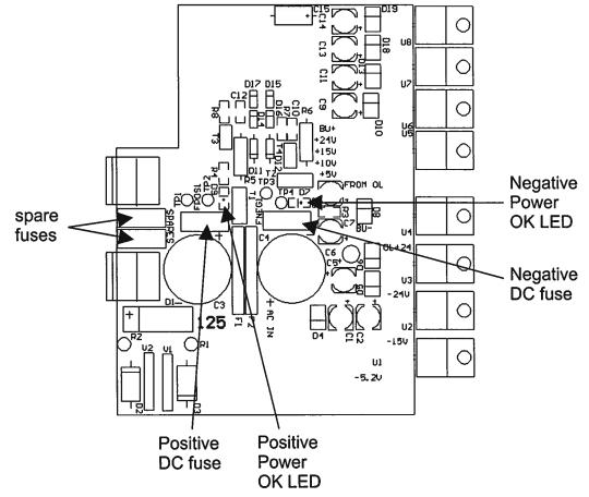
The positive fuse and one of the spare fuses on this circuit board are 2A slow-blow fuses, Littlefuse part number R45202.5. (This fuse can be ordered from Digikey, www. digikey.com. The Digikey part number is F1346CT-ND). The negative fuse and the second spare fuse are 0.5A slow-blow fuses (Littlefuse R452.500, Digikey part number F1341CT-ND).
