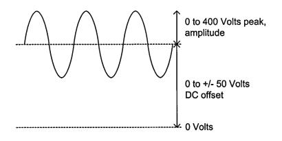
The total output (i.e., the sum of the offset and the amplitude) may not exceed ±400V.
