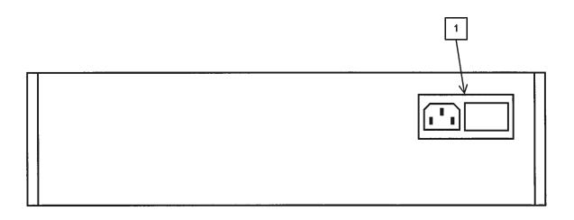
1. <u>AC POWER INPUT</u>. A three-pronged recessed male connector is provided on the back panel for AC power connection to the instrument. Also contained in this assembly is a slow-blow fuse and a removable power selector card that can be removed and repositioned to switch between 110-120V AC in and 220-240V.
