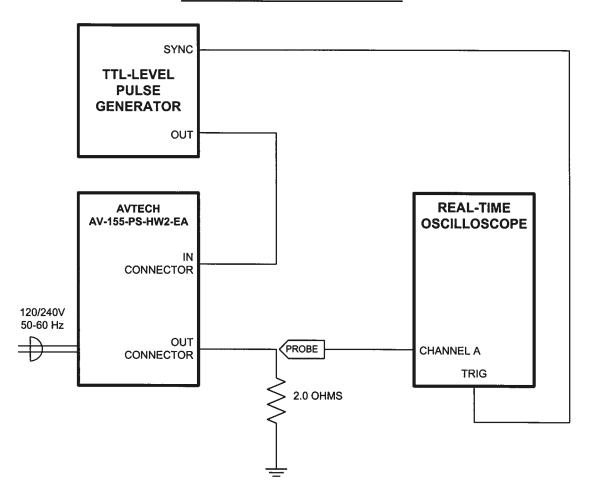
The input and output waveforms for the unit are below. Note that the unit operates as a pulsed constant current source and for that reason the load resistance should be less than 2.5 Ohms (to avoid saturating the output stage) and the load inductance must be exceedingly low (to avoid inductive spikes on the transitions).
