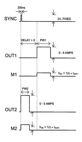
Basic Output Pulses for Delay > 0
