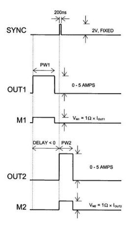
Basic Output Pulses for Delay < 0
