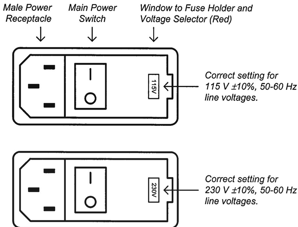
If the voltage selector is not set for to proper voltage, use a small flat-head screwdriver to pry open the voltage selector panel, as shown below:
