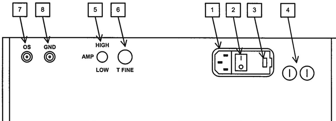
1. **AC POWER INPUT.** An IEC-320 three-pronged recessed male socket is provided on the back panel for AC power connection to the instrument. One end of the detachable power cord that is supplied with the instrument plugs into this socket.
