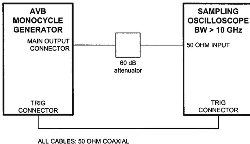
The bandwidth capability of components and instruments used to display the pulse generator output signal (attenuators, cables, connectors, etc.) should exceed 10 GHz.
