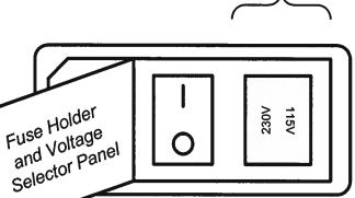
Once the panel is open, the red fuse holder / voltage selector should be visible. To change the voltage setting, pull out the red fuse holder / voltage selector and rotate it so that the proper voltage marking will shown through the panel window. Re-install the red fuse holder / voltage selector, and close the panel.
