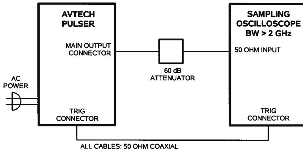
The attenuators are required to prevent damage to the sampling oscilloscope. A 60 dB attenuator with sufficient voltage rating should be used on the main output. Avtech suggests the Midwest Microwave ATT-0527-XX-SMA-07 family of fixed 12 GHz, 20 Watt attenuators for use with the AVB2-TC-C.
