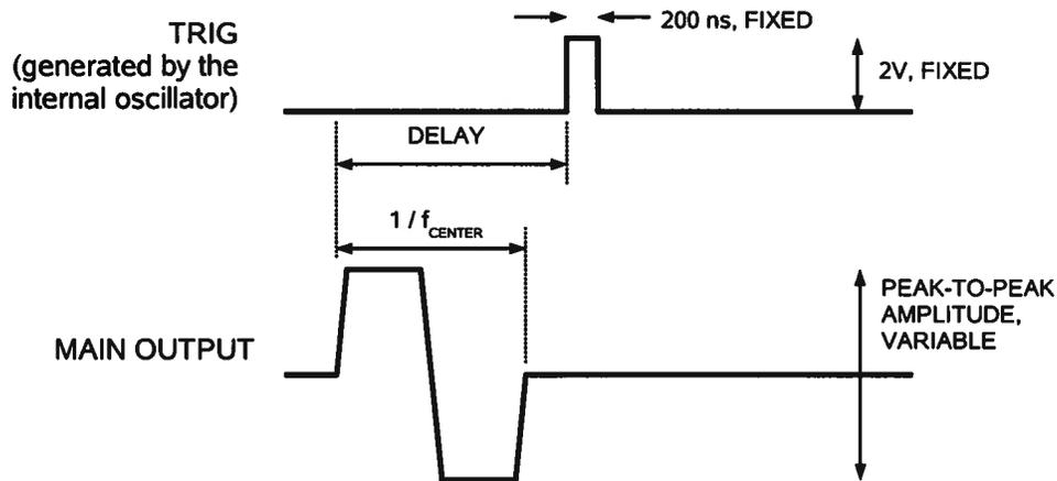
When triggered externally, the TRIG connector acts as an input. The delay controls do not function in this mode. This illustrated below:
