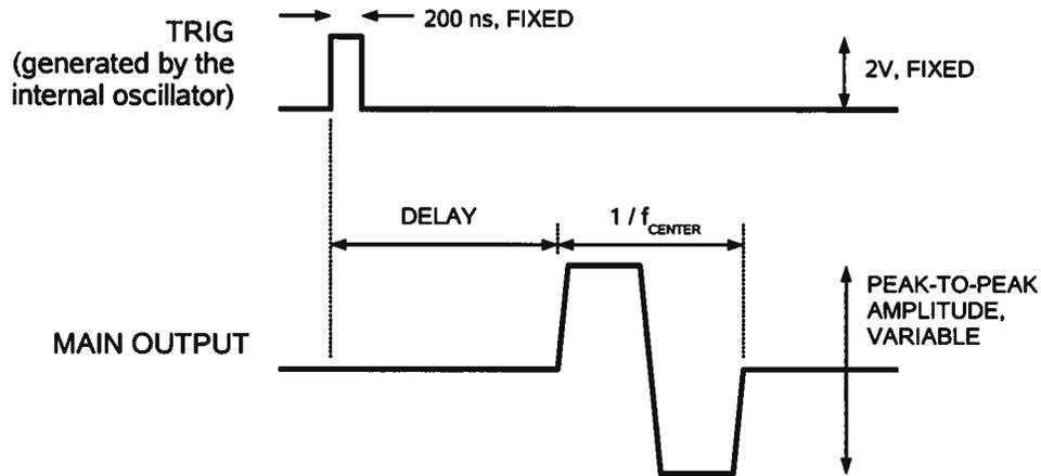
When the ADVANCE/DELAY switch is set to "DELAY", the TRIG output occurs after the main output. This illustrated below:
