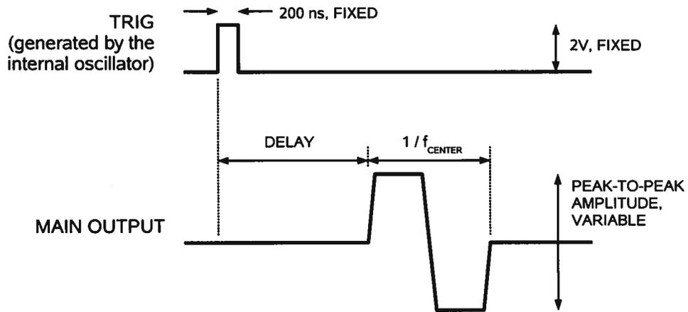
When the ADVANCE/DELAY switch is set to "DELAY", the TRIG output occurs after the main output. This is illustrated below:
