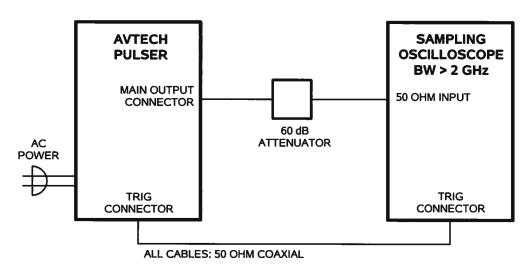
The attenuators are required to prevent damage to the sampling oscilloscope. A 60 dB attenuator with sufficient voltage rating should be used on the main output.
