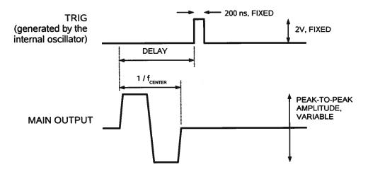
When triggered externally, the TRIG connector acts as an input. The delay controls do not function in this mode. This illustrated below:
