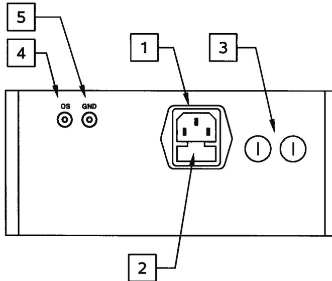
1. **AC POWER INPUT.** An IEC-320 C14 three-pronged recessed male socket is provided on the back panel for AC power connection to the instrument. One end of the detachable power cord that is supplied with the instrument plugs into this socket.
