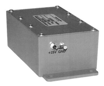
The +15V input terminal is protected with a 1N4746A Zener diode, which will fail as a short if an excessive positive voltage (> 18V), or a negative voltage, is applied to the terminal.
