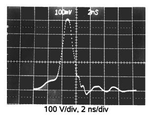
Capacitive loading will inevitably introduce some amplitude loss and transient distortions, as shown below for the example of 20 pF in parallel with 50 Ohms, located at the end of a 24" length of coaxial cable:
