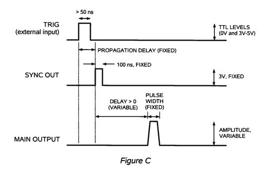
As before, if the delay is negative, the order of the SYNC and OUT pulses is reversed.
