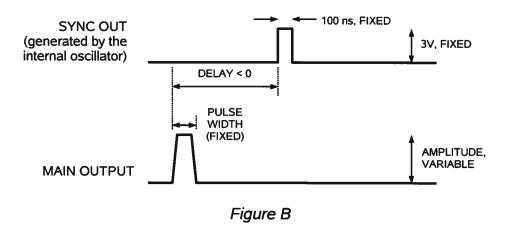
The next figure illustrates the relationship between the signal when an external TTL-level trigger is used:
