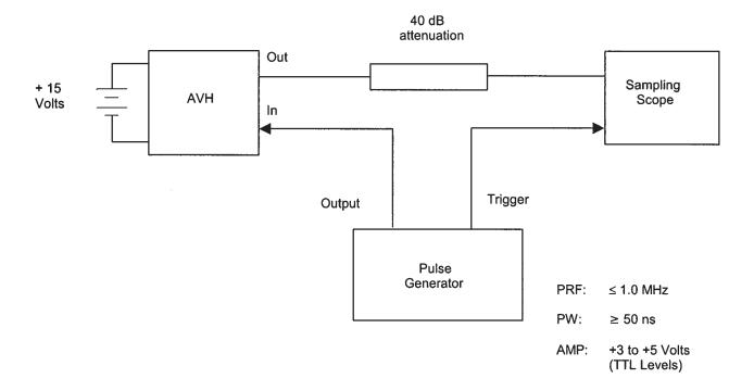
Power line: 15 Volts/0.2 Amps DC, shielded twisted pair, < 3 meters
