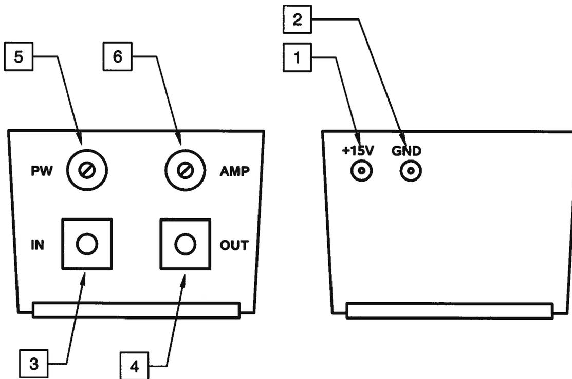
1. +15V POWER Input. Apply +15V prime power to this solder terminal.
