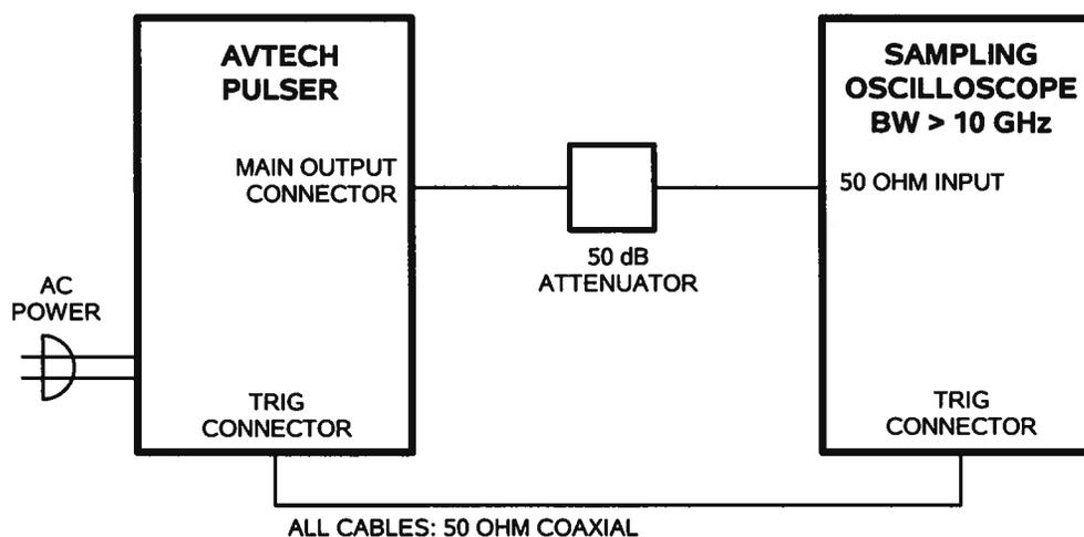
The attenuators are required to prevent damage to the sampling oscilloscope. A 50 or 60 dB attenuator with sufficient voltage rating should be used on the main output. Factory tests are conducted using several Midwest Microwave 10 dB and 20 dB attenuators (models ATT-0444-10-SMA-02 and ATT-0444-20-SMA-02, respectively) connected in series.
