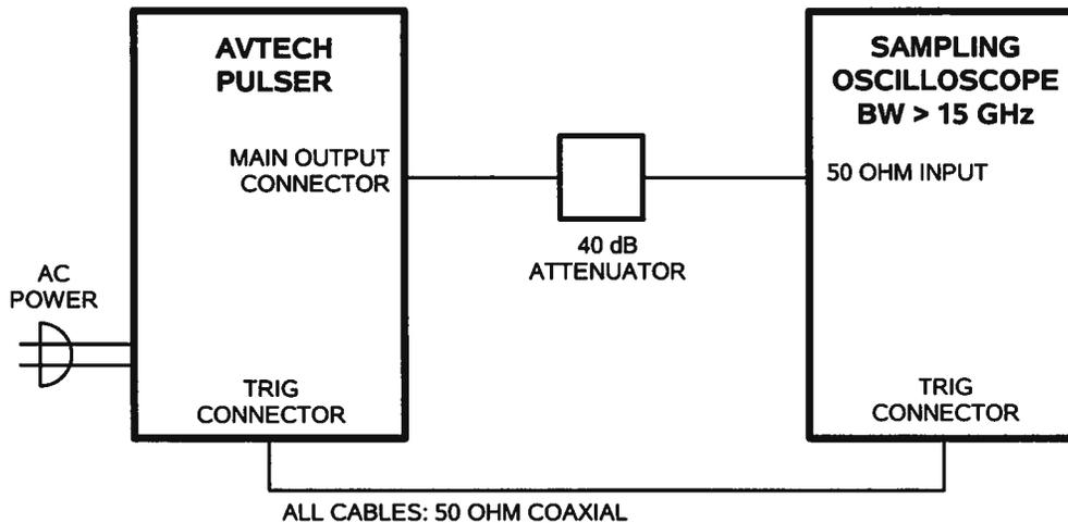
The attenuators are required to prevent damage to the sampling oscilloscope. A 20-40 dB attenuator with sufficient voltage rating should be used on the main output. Factory tests are conducted using several Midwest Microwave 10 dB and 20 dB attenuators (models ATT-0444-10-SMA-02 and ATT-0444-20-SMA-02, respectively) connected in series.
