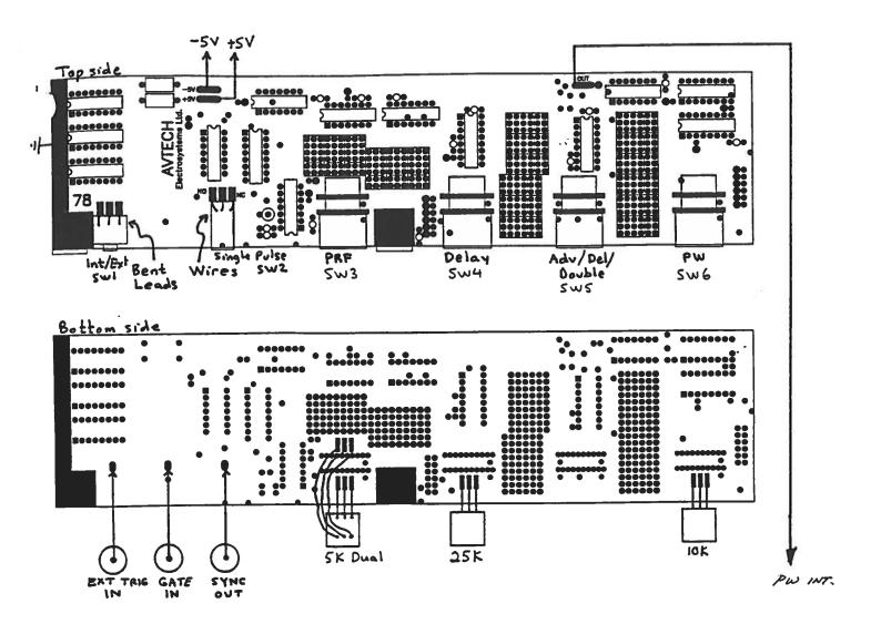
SW1 - MTA-106D-WW SW2 - pushbufton SW3, SW4, SW6 - 71ADF 36-02-1-ATN SW4 - 71ADF 36-02-2-ATN
