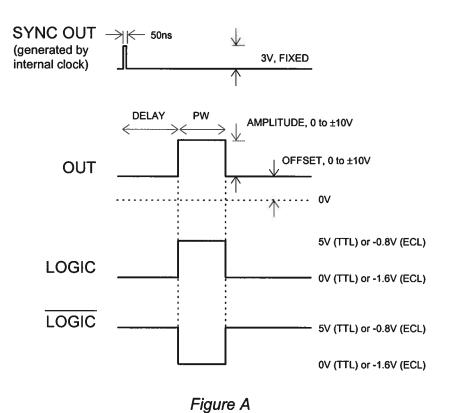
If the delay is negative, the order of the SYNC and OUT pulses is reversed:
