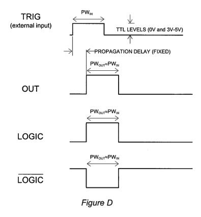
The delay, pulse width, and frequency (when in the internal mode), of the OUT pulse can be varied with front panel controls or via the GPIB or RS-232 computer interfaces.
