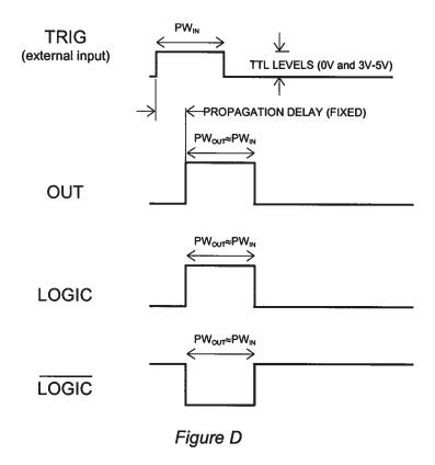
The delay, pulse width, and frequency (when in the internal mode), of the OUT pulse can be varied with front panel controls or via the GPIB or RS-232 computer interfaces.
