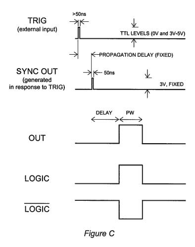
As before, if the delay is negative, the order of the SYNC and OUT pulses is reversed.
