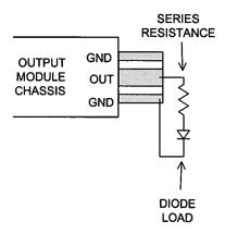
The load should be connected between the OUT and GND terminals using very short leads (<5.0 cm, and preferably < 0.5 cm). Severe inductive voltage spikes will result from any series inductance (Lenz's Law). Take care to ensure that during soldering the OUT conductor is not shorted to the chassis. Use minimal heat when soldering to avoid delaminating the metal pads.
