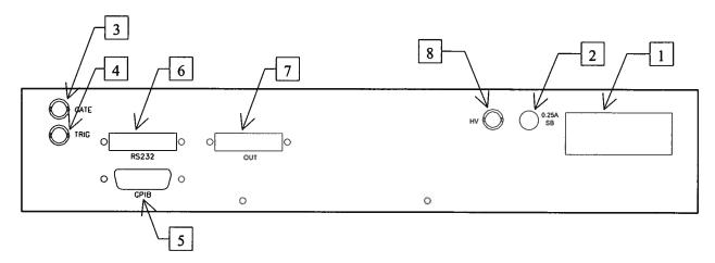
Note: Dual polarity "-PN" models will have one "OUT" and "HV" connector for each polarity.
