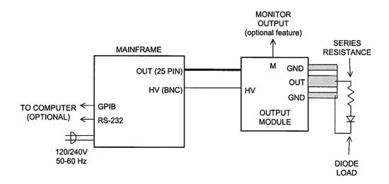
The loads can be connected (soldered) to the microstrip transmission line that protrudes from the output module. The lead lengths must not exceed several centimeters or severe inductive voltage spikes will result (as predicted by Lenz's Law.)
