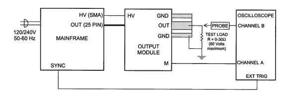
The equipment should be connected in the general fashion shown above (see page 8 also). For dual-polarity instruments, both output modules should be connected, with the positive output module connected to the "HV P" and "OUT P" connectors, and the negative output module connected to the "HV N" and "OUT N" connectors.
