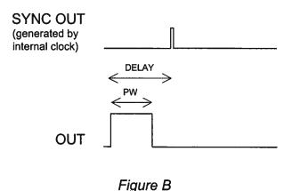
The next figure illustrates the relationship between the signal when an external TTL-level trigger is used:
