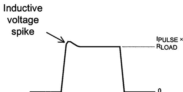
Attaching a current transformer (for measuring current waveforms) can add significant inductance, because of the necessary wire length that must be fed through the transformer. (The Pearson 2878 requires approximately 1.5".) For this reason it is recommended that the optional self-contained current transformer ("M") be used.
