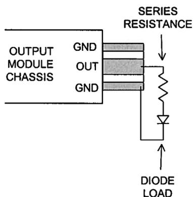
The load should be connected between the OUT and GND terminals using very short leads (<5.0 cm, and preferably < 0.5 cm). Severe inductive voltage spikes will result from any series inductance (Lenz's Law). Take care to ensure that during soldering the OUT conductor is not shorted to the chassis. Use minimal heat when soldering to avoid delaminating the metal pads.
