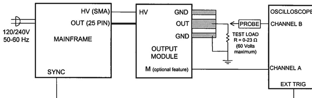
The equipment should be connected in the general fashion shown above (see page 8 also). For dual-polarity instruments, both output modules should be connected, with the positive output module connected to the "HV P" and "OUT P" connectors, and the negative output module connected to the "HV N" and "OUT N" connectors.
