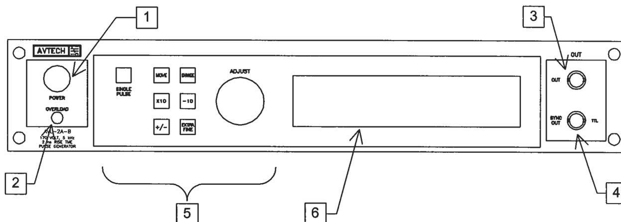
1. **POWER Switch.** The POWER push button switch applies AC prime power to the primaries of the transformer, turning the instrument on. The push button lamp (#382 type) is connected to the internal +15V DC supply.
