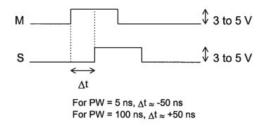
As the pulse width is varied over its full range ∆t should vary from about -50ns to approximately +50 ns. If the waveforms at the M and S pins do not resemble the above, then the -T101 module is defective and should be replaced. If the waveforms do resemble the above then the -PG module is at fault and should be replaced. Replacement modules should be ordered by part number (eg. AVL-2A-PG) from Avtech.
