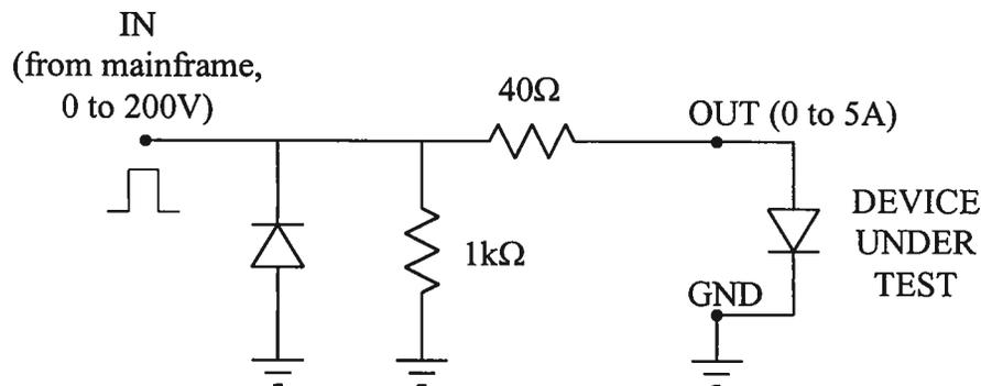
*Output Module Functional Equivalent Circuit*
