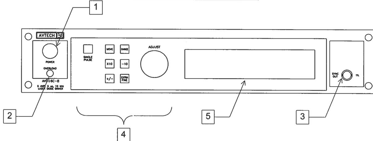
1. **POWER Switch.** The POWER push button switch applies AC prime power to the primaries of the transformer, turning the instrument on. The push button lamp (#382 type) is connected to the +15V DC supply.
