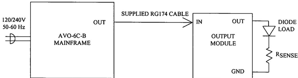
If  $R_{SENSE}$  is not used, connect the diode cathode directly to the GND terminal. (The diode is shown oriented for a positive output current.)
