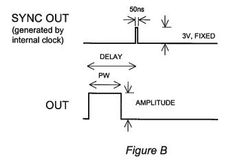
The next figure illustrates the relationship between the signal when an external TTL-level trigger is used:
