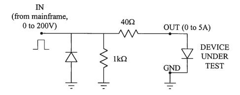
Output Module Functional Equivalent Circuit
