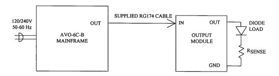
If R<sub>SENSE</sub> is not used, connect the diode cathode directly to the GND terminal. (The diode is shown oriented for a positive output current.)
