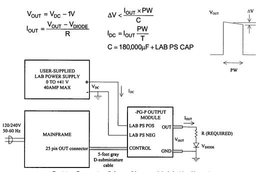
Positive Connection Scheme (Negative Module Not Shown)
