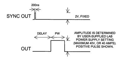
Figure 4 - Basic Output Pulses
