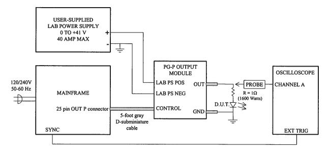
For use with the PG-N output module (i.e., negative output, -N and -PN models):
