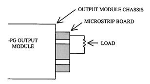
Take care to ensure that during soldering the OUT conductor is not shorted to the chassis. Also, use minimal heat when soldering.
